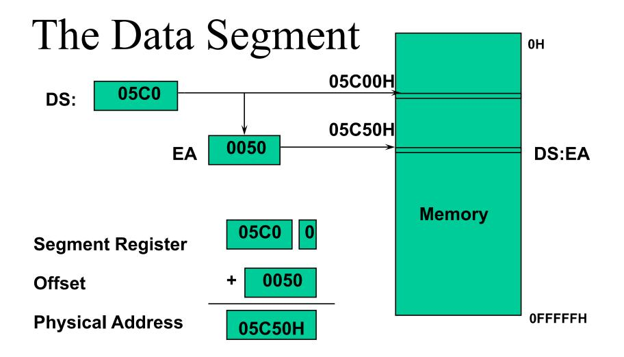
Data is usually fetched with respect to the DS register. The effective address (EA) is the offset. The EA depends on the addressing mode.
