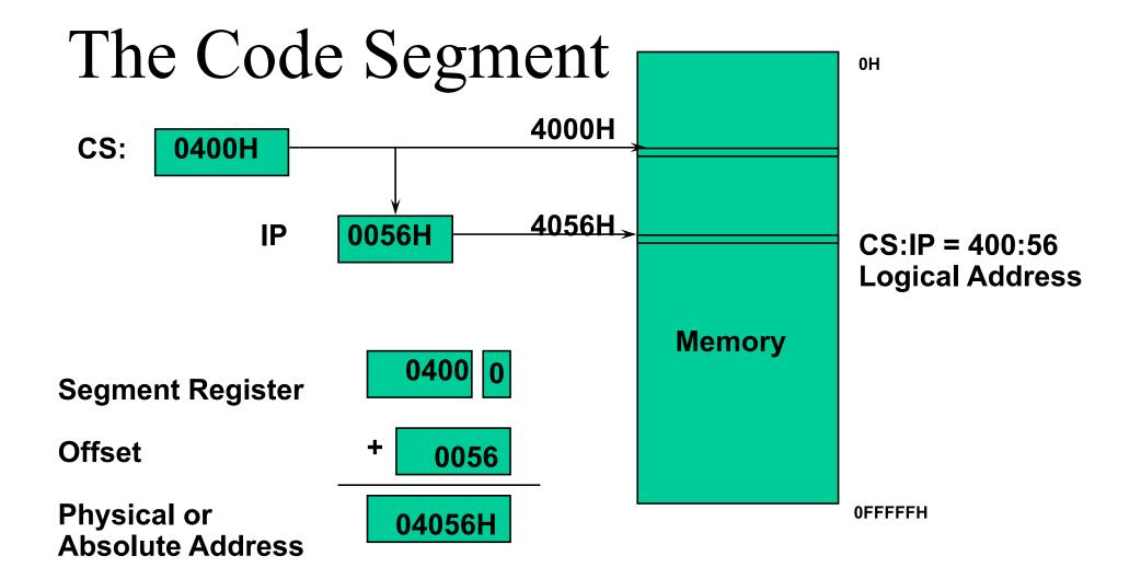
The offset is the distance in bytes from the start of the segment. The offset is given by the IP for the Code Segment. Instructions are always fetched with using the CS register.
